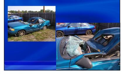
Roof intrusion over DR = 35 cm (14 in) Roof intrusion over LR cargo area = 53 cm (21 in)
